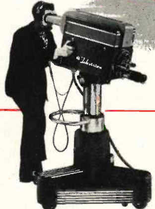
RCA Studio Pedestal, Type MI-26035. Lowers and raises camera manually—rolls quietly, steers readily by means of a circular handle around the pedestal base. RCA Friction Head, type MI-26205, provides horizontal panning action and a vertical tilting movement—lock-holds the camera in any position. The camera includes the intercommunication circuits.
